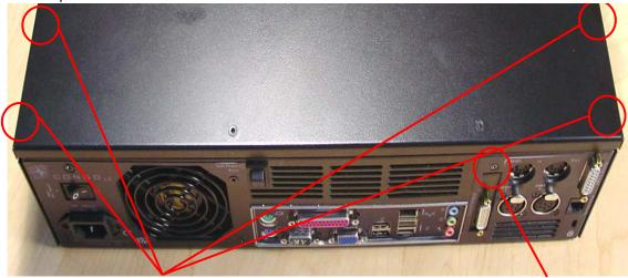
Remove these screws (located on side of chassis)
