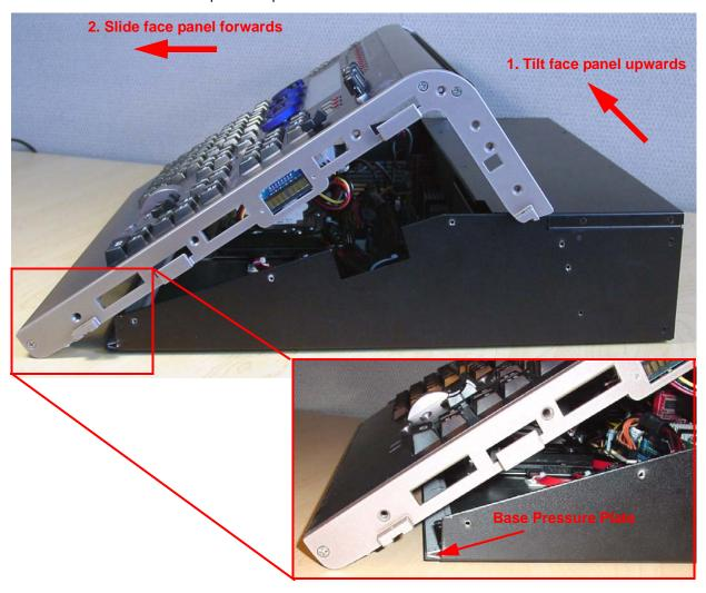
Step 8: Rest the face panel off to the left side of the base unit. (the side with the DMX connectors) There is no need to remove the face panel cables when replacing the video card.
